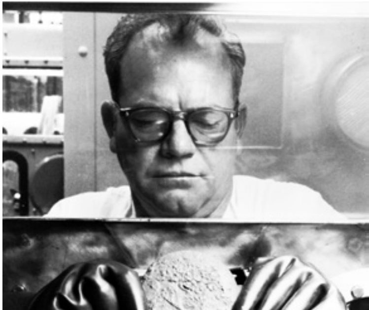
A technician at Rocky Flats working with a Plutonium "puck" prior to it being machined.
