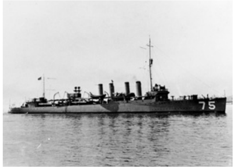
The Wickes-class destroyers were a class of 111 destroyers built by the United States Navy in 1917-19. They formed the "four-stack" type. Only a few were completed in time to serve in World War I, including USS Wickes, the lead ship of the class.
